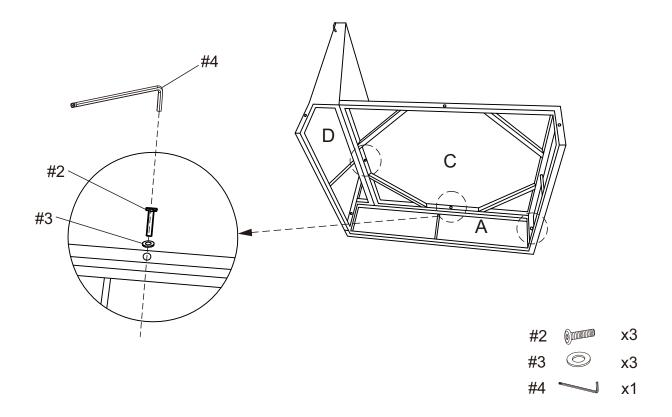
Step 3. Attach left arm panel (part B) to back panel (part D) and seat panel (part C) using long bolts (part #2), flat washers (part #3) and allen wrench (part #4).
