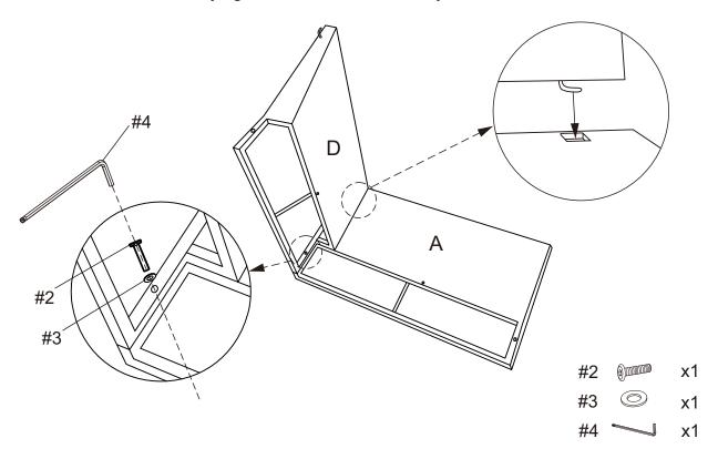
Step 2. Attach seat panel (part C) to right arm panel (part A) and back panel (part D) using long bolts (part #2), flat washers (part #3) and allen wrench (part #4).
